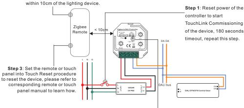
Step 4: There shall be indication on the remote and LED indicator flashes 3 times for successful reset.
